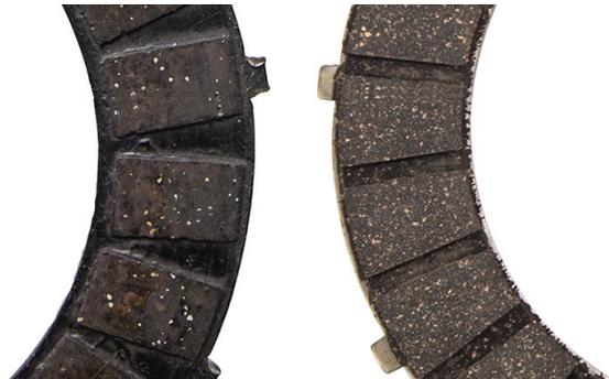
The image on the left shows damage from wear, and the image on the right show the protection provided by Performance Plus.
