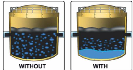
Our blend of additives will force any water contamination to the system to settle to the bottom of the sump so it can be easily drained off to protect the system.
